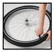
First, deflate your tire, and then use the lever (or the back of a metal spoon) provided in your box to separate the tire from the rim.
