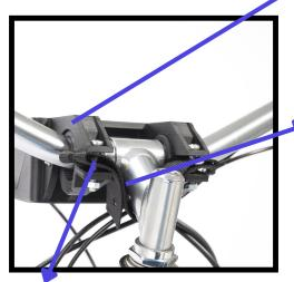
Rubber: Rubber provides durability for your bracket arms. Secure the rubber pieces onto the **upper leg** as shown in the picture.
