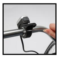
After removing the grip, install the throttle and then tighten it securely with a number 3 Allen key.
