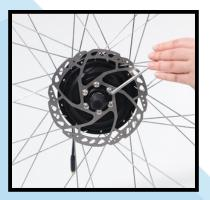
Remove the bolts on the left side of the motor to detach the plate. Install your new disc brake rotor in its place. When positioning the motor on the fork, align the disc brake rotor with the brake mechanism for proper seating.
