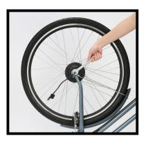
Attention: In this step, for 100mm motors, the motor cable should be on the **right** side, and for 74mm motors, it should be on the **left** side.
