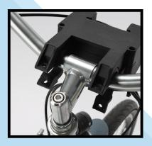
Detach the bolts and cord attached to the bracket arms. Attach the **rubber** pieces that come with the bracket onto the upper arms.
