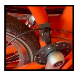
If your sensor does not reach the disk, place the rubbers from your box behind the sensor as shown in the right picture. (This is necessary for Brompton)
