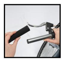
For the "106DX Throttle", "103X Throttle", and "On/Off Switch" accessories, you will need to remove the grip. To make grip removal easier, you can use "cologne".
