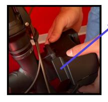
Firmly position the bracket onto the "Mounting Part".
