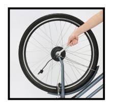
Attention: In this step, for 100mm motors, the motor cable should be on the **right** side, and for 74mm motors, it should be on the **left** side.
