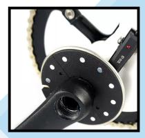
Connect the connectors according to the cable diagram shown above. Once the installation is complete, when you rotate the pedal with the battery connected, the light on the sensor should be blinking. If you cannot observe the light, it indicates an error in the installation.
