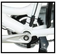
For installation, first determine a position where the "+" sign on the sensor can touch the magnets on the disc after mounting. Then mount it to the location shown in the picture using cable ties.
