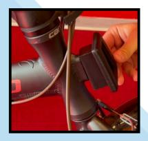
Place the front attachment device onto the front bag connection point of your bicycle.
