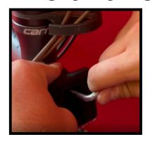
Install the mounting bolts from your box to secure the "Mounting Part" using a 4mm Allen key.
