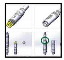
Connect the motor cable coming out of the bracket to the connection point on the motor.
